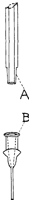
A, ground glass Luer adapter which fits into B; B, a hypodermic needle. Drawing is actual size.
